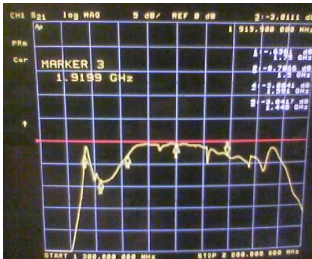
Coupling: antennas held face-to-face
