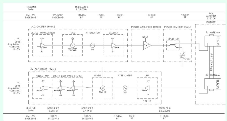
Coffee Can Radar Block Diagram
