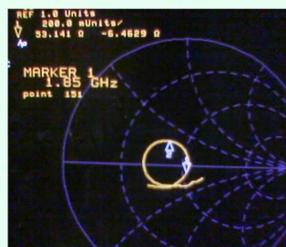
Smith chart of open-ended circular waveguide antenna
