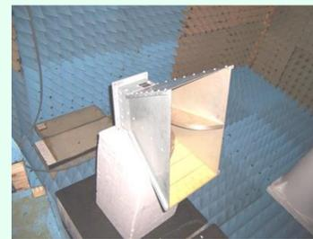
500MHz..6GHz Anechoic Range Antenna for reference testing
