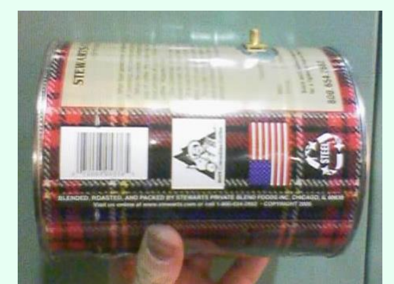
Coffee can 1.5–2.0GHz as open-ended circular waveguide antenna—female SMA attached to 1/4 wavelength probe for TE mode excitation
