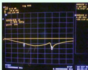
S11 plot of open-ended circular waveguide antenna prototype
