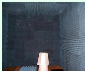
Anechoic chamber rotary antenna-under-test location
